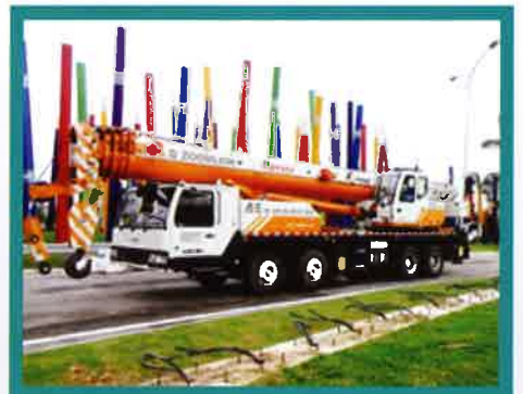
MOBILE CRANE (55 TONS)
